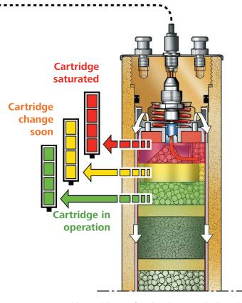
An additional layer of molecular sieve (red marking) allows a time buffer of 3-7 hours after the first warning message.
